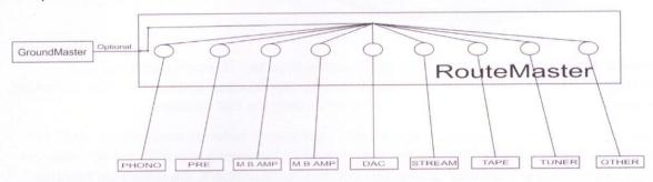
RouteMaster accepts grounding reference connections from up to nine system components. Simply identify a spare input and connect it with the appropriate Ultra Connect cable. For the very optimum results all RouteMaster UltraConnects should be the same length and hence resistance.
